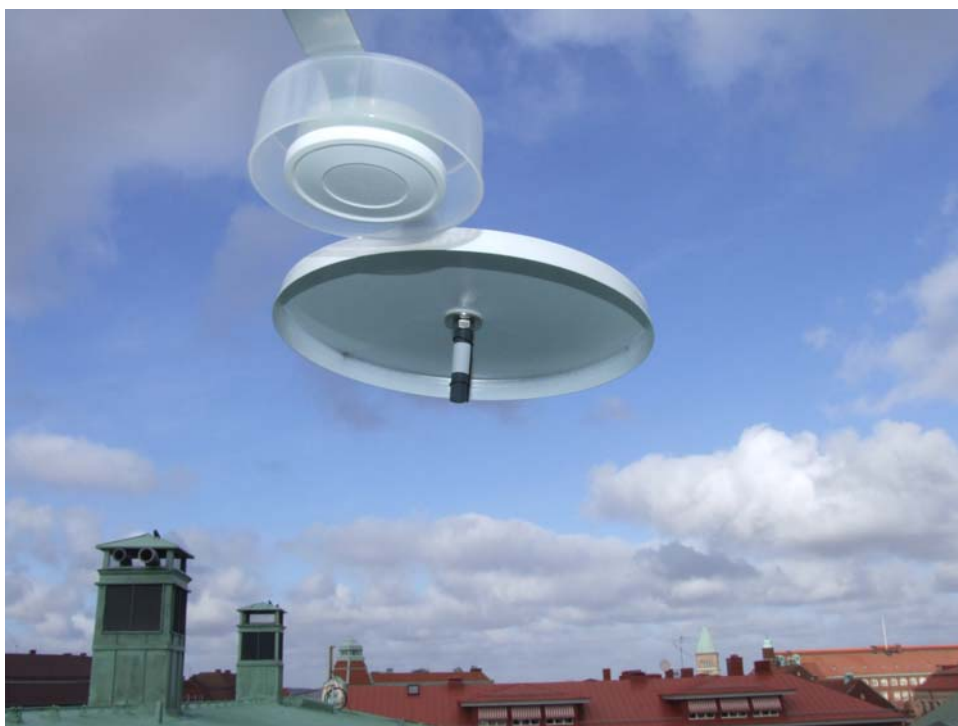
Figure 3. Photo of the passive sampler for fine particles (front) and the sampler for larger particles (farther).
