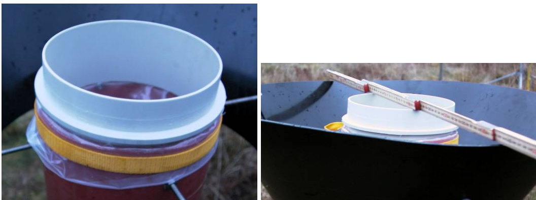
Figure 5. A rim has been constructed of a polypropylene tube. It is fitted into the sampling tube and levelled with the rain shield.
