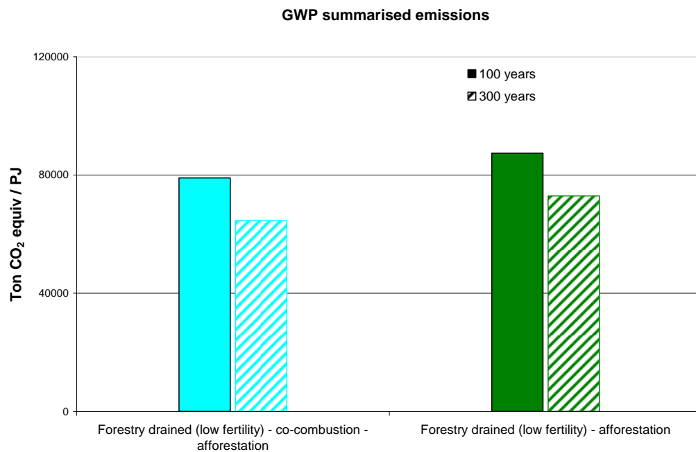
Figure 12 Accumulated emissions summarised by GWP after 100 years and 300 years for energy peat utilisation from drained forested peatlands with low fertility, with and without the effect of co-combustion included.
